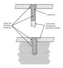
**Lineally Applied (21)** - A bonded detail is considered to be lineally applied when it is a long thin part typically with a width of 2.0" or less and the surface area is spread out in a long, narrow band. Examples of bonded details that commonly meet this definition include, but are not limited to, rub strips/trims, edge trim/non-metallic, exterior wire raceways, felt, kickstrips, metal and plastic bracket, hook and loop fastener, and grommets.
